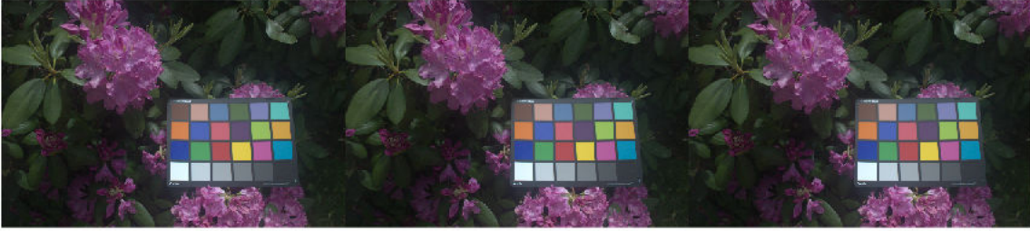
sRGB Image Using PCS, raw2rgb Function, and Transformation Matrix (Left to Right)
